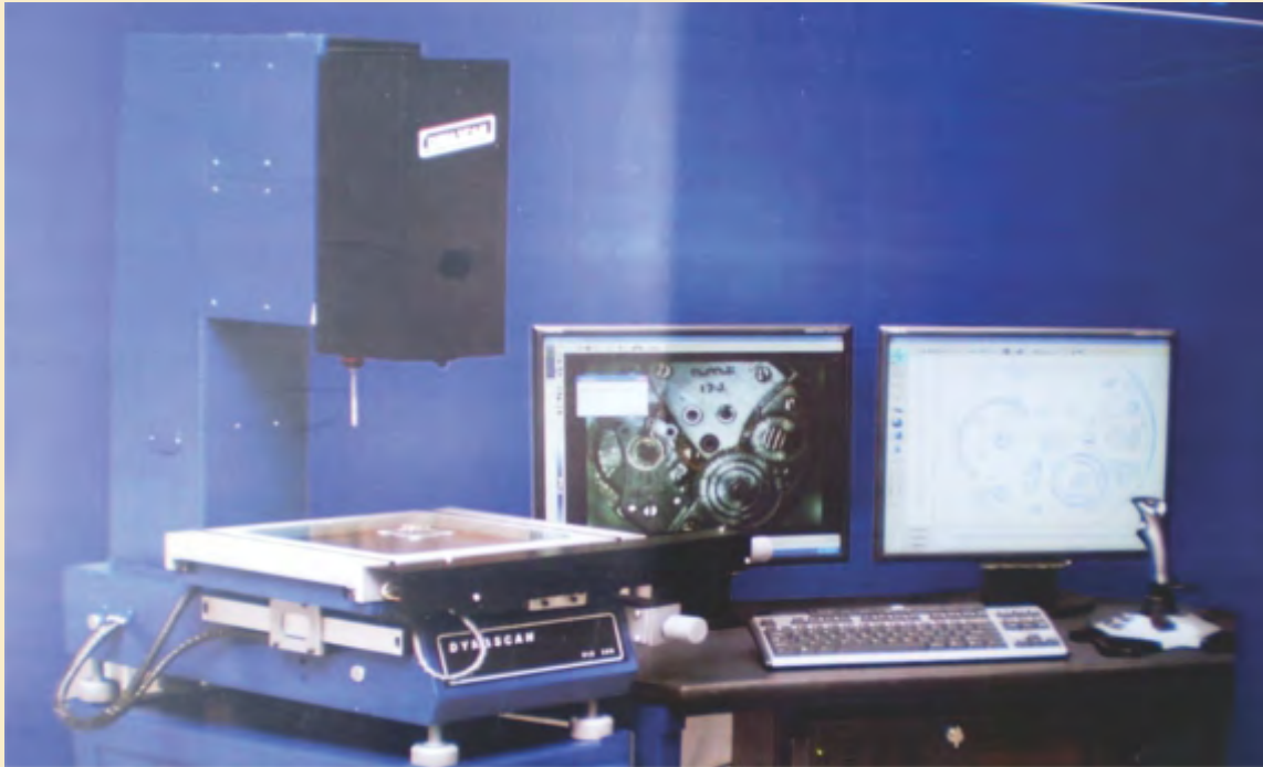
IMAGE PROCESSING MACHINE WITH GRANITE BASE WITH COLUMN Material supplied by GMT : Granite base with column
